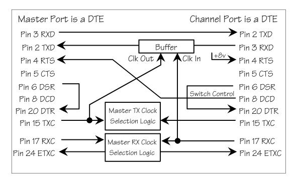
Master DTE / Sub-Channel DTE Interface Flow Diagram
